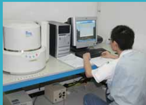
Fluorescent X-ray analysis of the RoHS Directive banned substances
