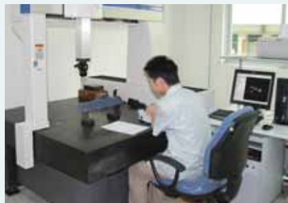
Dimension measurement is performed in the shipping inspection, using a three-dimensional measuring system.
