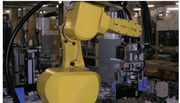
Container assembling robot
