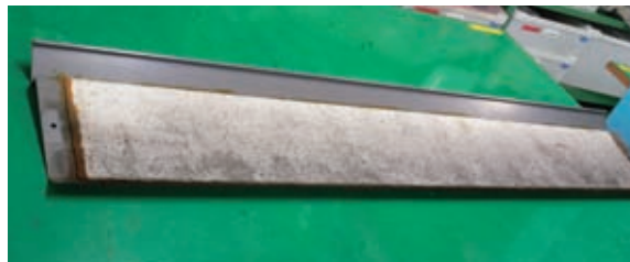
Parts before replacement (containing asbestos)
