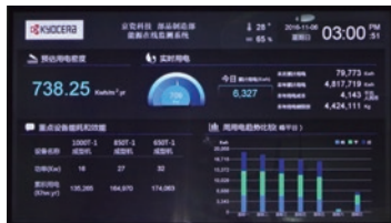
Monitor screen for the energy management system
