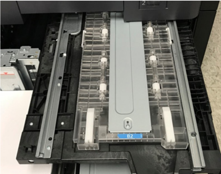
Misfeed areas are easily identified inside the machine with blue labels and numbers.
