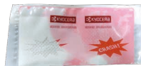
Shock gauge after impact; colour appears due to rupture of internal ink bag
