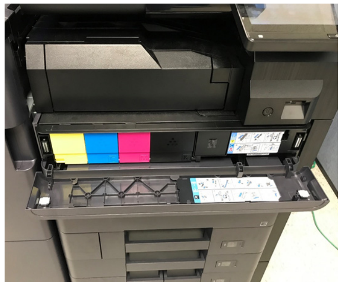
The process for replacing toner is simple and clean. Only when the container is empty will the device notify the user to open the front panel and make the replacement, helping to prevent premature replacement of toner. Guidance at the control panel is extensive and includes text, graphics, animation, and video.
