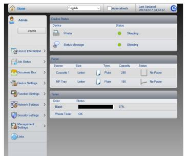
Command Center RX provides administrators with information about the unit and lets them handle tasks such as changing device settings, viewing device status and monitoring toner and paper supplies. It also allows administrators to configure email alerts that can be sent to up to three recipients for error conditions, including paper jam, cover open and add toner/paper.
