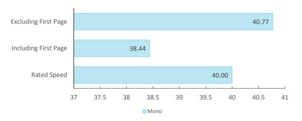
Print speed is tested using BLI's Monochrome Test Original with 6% page coverage. The test page is printed in a quantity equal to double the vendor's rated print speed for the device in each mode tested (e.g., if the vendor's rated print speed is 20 ppm, 40 pages are printed). The unit's print speeds were tested using the PCL 6 driver.
