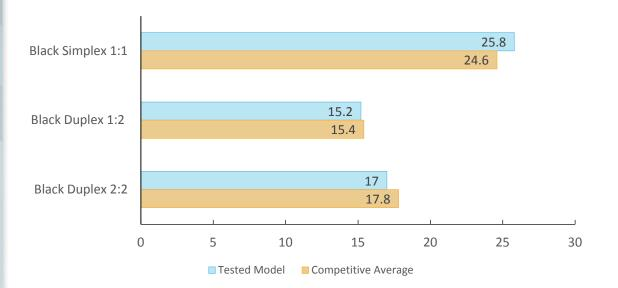
Single-set copy speed is tested using a 10-page black document. Timing begins as the start button is pressed, pages are scanned through the document feeder and timing ends when the last page of a single-set of the document exits the device.
