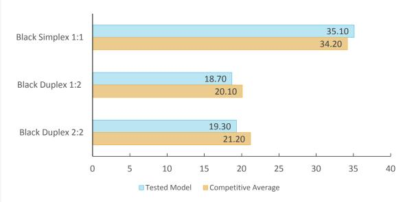
Copy speed is tested using a 3-page and a 10-page black document. BLI obtains the overall speed by averaging the tested speed for each run length (1, 5, 10 and 20 sets).
