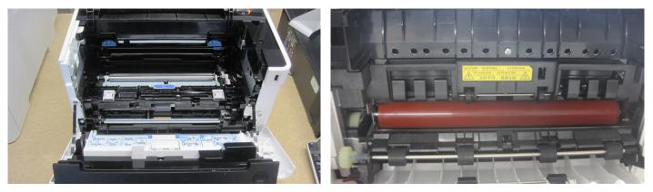
Users can expect to have to change consumables a little more frequently than they would with competitive models tested to date, according to BLI's calculations. Removing misfeeds, either at the front (shown left) or at the rear of the device (shown right), is extremely easy. If accessed at the front, the process unit (drum and developer) needs to be pulled out, but the surface of the drum is not exposed to any risk of damage during removal.
