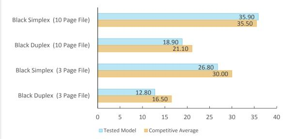
Print speed is tested using a 3-page and a 10-page black document. BLI obtains the overall speed by averaging the tested speed for each run length (1, 5, 10 and 20 sets). The unit was tested using the PCL 6 driver.
