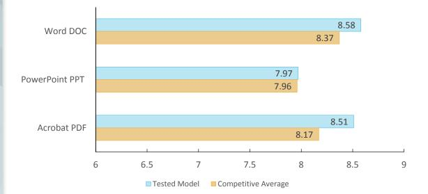
First-print time indicates the time it took to process, image and deliver a single-page test document to the output tray. Files tested include a Word document (.doc; black text), a PowerPoint slide (.ppt; colour graphics and text) and an Acrobat file (.pdf; black text and graphics). The unit's print speeds were tested at the default 600 dpi using the PCL 6 driver.
