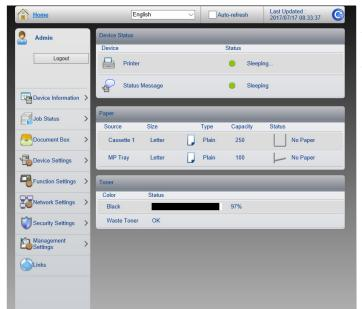
Command Center RX provides administrators with information about the unit and lets them handle tasks such as changing device settings, viewing device status and monitoring toner and paper supplies. It also allows administrators to configure email alerts that can be sent to up to three recipients for error conditions, including paper jam, cover open and add toner/paper.
