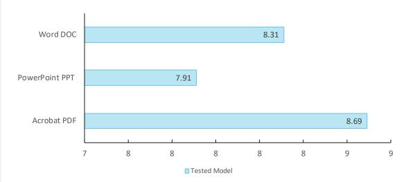
First-print time indicates the time it took to process, image and deliver a single-page test document to the output tray. Files tested include a Word document (.doc; black text), a PowerPoint slide (.ppt; color graphics and text) and an Acrobat file (.pdf; black text and graphics). The unit's print speeds were tested at the default 600 dpi using the PCL 6 driver.
