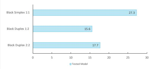
Single-set copy speed is tested using a 10-page black document. Timing begins as the start button is pressed, pages are scanned through the document feeder and timing ends when the last page of a single-set of the document exits the device.
