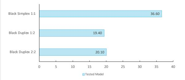
Copy speed is tested using a 10-page black document. BLI obtains the overall speed by averaging the tested speed for each run length (1, 5, 10 and 20 sets).
