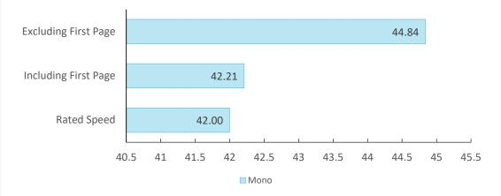
Print speed is tested using BLI's Monochrome Test Original with 6% page coverage. The test page is printed in a quantity equal to double the vendor's rated print speed for the device in each mode tested (e.g., if the vendor's rated print speed is 20 ppm, 40 pages are printed). The unit's print speeds were tested using the PCL 6 driver.
