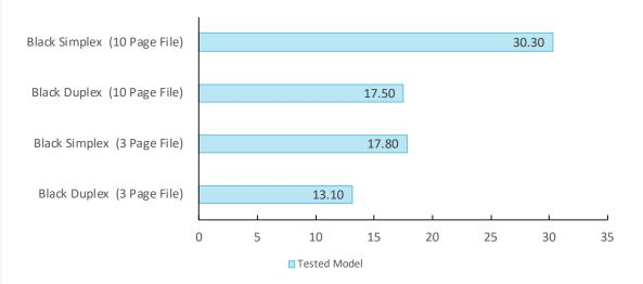
Single-set speed is tested using a 3-page and a 10-page black document. The unit was tested using the PCL driver.
