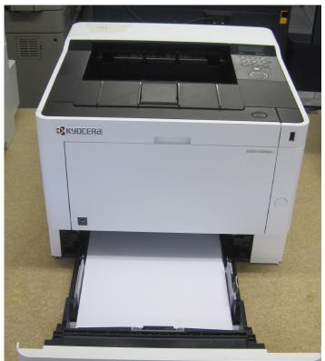
Adjusting the drawer for different-size paper is simple; the length and width guides move in sync. Loading letter-size media is very easy: users press the tab at the front of the unit, pull out the drawer, load the paper and press down on the spring-loaded ramp before sliding the tray back in.
