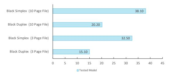
Print speed is tested using a 3-page and a 10-page black document. BLI obtains the overall speed by averaging the tested speed for each run length (1, 5, 10 and 20 sets). The unit was tested using the PCL 6 driver.
