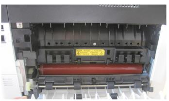
Misfeed access is either at the front (shown above) or at the rear of the device. If accessed at the front, the drum unit needs to be removed, but the surface of the drum is not exposed to any risk of damage during removal.
