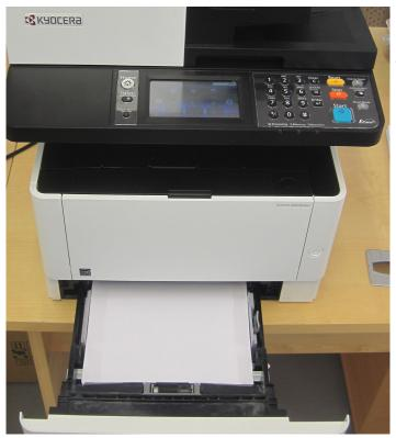
Buyers Lab technicians noted that loading paper trays is easy, with sliding paper guides, which move in sync. As is typical of models in this class, paper sizes must be confirmed on the touchscreen.
