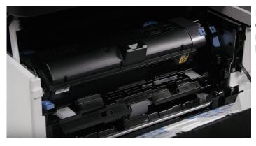
Procedures for replacing toner are easy. Although it can't be replaced while the unit is running, the cartridge is accessible from the front and lifts out easily after a blue lever on the left has been released.
