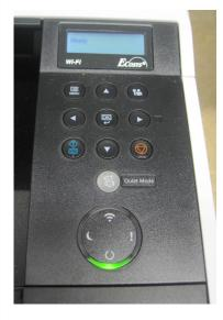
The KYOCERA ECOSYS P2040dw has a very simple, intuitive control panel design with a small LCD display, an alphanumeric keypad and up/down and left/right keys for menu navigation.
