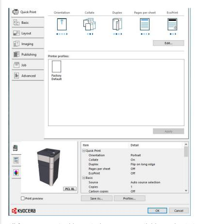
All features required by typical users are available on the Quick Print screen of the driver, and its layout is clear and intuitive.
