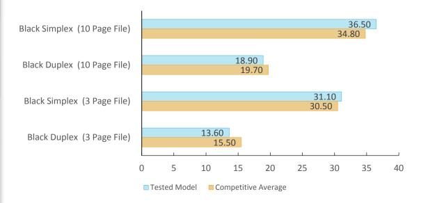
Average print speed is tested using 3-page and 10-page black documents. BLI obtains the overall speed for each mode by averaging the tested speed for each run length (1, 5, 10 and 20 sets). The unit was tested using the PCL driver.
