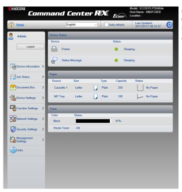
Command Center RX provides users at the desktop with a good level of feedback regarding the P2040dw, including device status, paper size, remaining paper and toner supplies.
