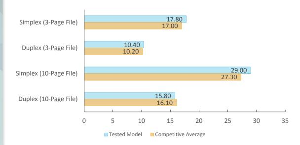
Single-set speed is tested using a 3-page and a 10-page black document. The unit was tested using the PCL driver.
