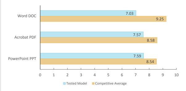
First-print time indicates the time it took to process, image and deliver a single-page document to the output tray. The unit's print speeds were tested at the default 600 dpi using the PCL driver.
