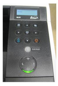
The KYOCERA ECOSYS P2040dw has a very simple, intuitive control panel design with a small LCD display, and up/down and left/right keys for menu navigation.
