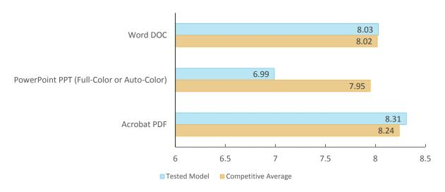
First-print time indicates the time it took to process, image and deliver a single-page document to the output tray. The unit's print speeds were tested at the default 600 dpi using the PCL driver.
