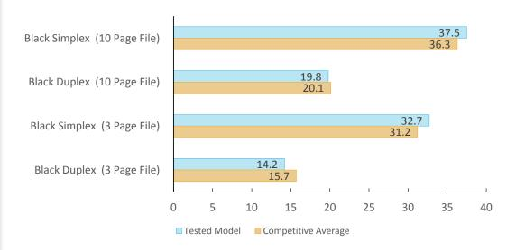
Average print speed is tested using 3-page and 10-page black documents. BLI obtains the overall speed for each mode by averaging the tested speed for each run length (1, 5, 10 and 20 sets). The unit was tested using the PCL driver.
