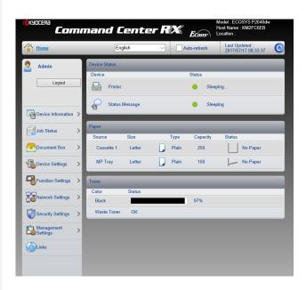
Command Center RX provides users at the desktop with a good level of feedback regarding the P2040dw, including device status, paper size, remaining paper and toner supplies.
