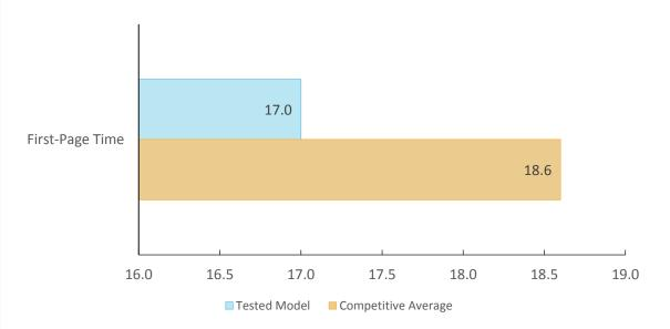
Device sits idle overnight; a single-page black Word document is sent to the device; first-print time indicates the time it took to warm up, process, image and deliver the test document to the output tray.
