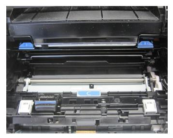
Misfeed access is either at the front (shown above) or at BLI technicians noted that loading paper trays is easy, the rear of the device. If accessed at the front, the drum with sliding paper guides, which move in sync. As is typunit needs to be removed, but the surface of the drum ical of models in this class, paper sizes must be conis not exposed to any risk of damage during removal.
