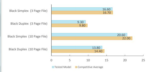
Single-set speed is tested using a 3-page and a 10-page black document. The unit was tested using the PCL driver.
