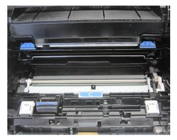
Misfeed access is either at the front (shown above) or at BLI technicians noted that loading paper trays is easy, the rear of the device. If accessed at the front, the drum with sliding paper guides, which move in sync. As is typunit needs to be removed, but the surface of the drum ical of models in this class, paper sizes must be conis not exposed to any risk of damage during removal.
