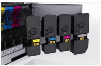
tray for different size paper; width paper guides slide can't be replaced while the unit is printing, the cartridges are accessible from the front. To replace toner, users must open the access door and release a blue lever on the left, and the cartridges lift out easily.
