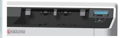
The KYOCERA ECOSYS P5026cdw has a very simple, intuitive control panel with a five-line LCD display, an alphanumeric keypad and up/down and left/right keys for menu navigation.
