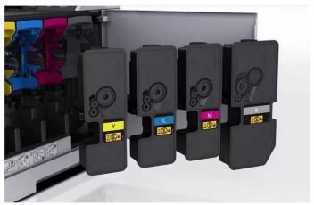
Loading media is straightforward, as is adjusting the Replacing toner is a mess-free process. Although they es are accessible from the front. To replace toner, users must open the access door and release a blue lever on the left, and the cartridges lift out easily.
