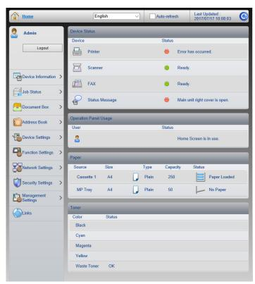
Command Center RX provides administrators with information about the unit and lets them handle tasks such as changing device settings, viewing device status and monitoring toner and paper supplies. It also allows administrators to configure email alerts that can be sent to up to three recipients for error conditions, including paper jam, cover open and add toner/paper.
