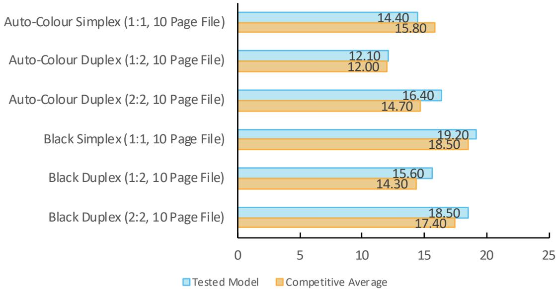
Single-set copy speed is tested using 3-page and 10-page mixed-colour and black documents. Timing begins as the start button is pressed, pages are scanned through the document feeder and timing ends when the last page of a single-set of the document exits the device.
