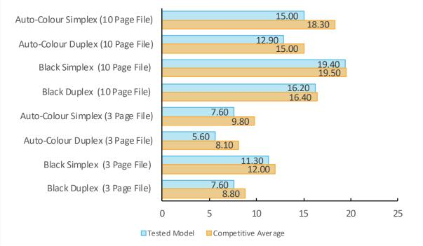
Single-set speed is tested using Buyers Lab's proprietary 3-page and 10-page testing documents. The unit was tested using the PCL driver.
