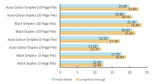
Speed is tested using Buyers Lab's proprietary 3-page and 10-page testing documents. Buyers Lab obtains the overall speed by averaging the tested speed for each run length (1, 5 and 10 sets). The unit was tested using the PCL driver.
