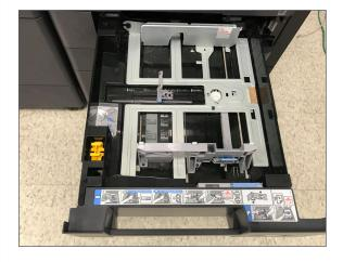
Both length and width guides slide in sync when adjusting paper size in the drawers and have blue locking tabs for easy view. The drawers also feature easy-to-see limit indicators for standard paper, envelopes, and small sizes. The soft close drawers make for no slamming of cassettes, and also pull our far enough for easy access in case of misfeed.
