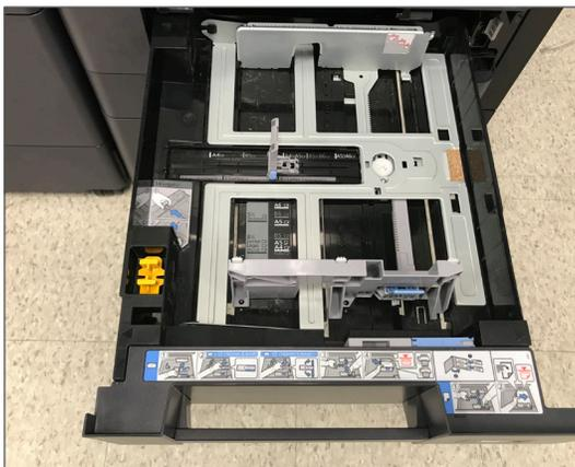
Both length and width guides slide in sync when adjusting paper size in the drawers and have blue locking tabs for easy view. The drawers also feature easy-to-see limit indicators for standard paper, envelopes, and small sizes. The soft close drawers make for no slamming of cassettes, and also pull out far enough for easy access in case of misfeed.
