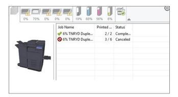
When the user sends a print job a pop up box appears showing all the paper trays and amounts of paper available in each drawer in percent increments, toner remaining in percent increments, and jobs in the print queue. Print job completion and deletion are supported. However, if the user closes out the pop up box during the print process, print job completion and/or deletion will not reappear.
