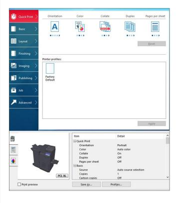
While an entire tab of the driver cannot be customized, users can save custom profiles that are stored as graphical icons via the Quick Print tab to allow programming of complex jobs in one click. Users can click on the Save As button on any of the tabs to save currently selected settings, name the new profile, and add a description for storage on the Quick Print tab.
