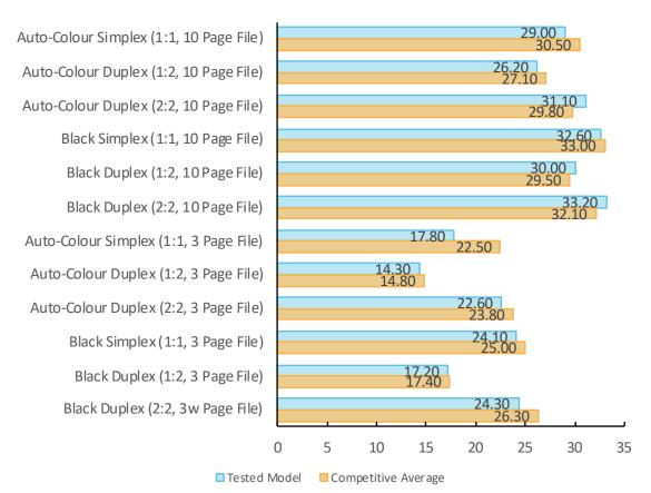
Copy speed is tested using 3-page and 10-page mixed-colour and black documents. Buyers Lab obtains the overall speed by averaging the tested speed for each run length (1, 5 and 10 sets).
