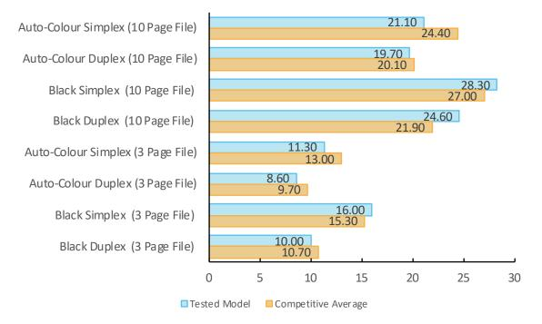
Single-set speed is tested using Buyers Lab's proprietary 3-page and 10-page testing documents. The unit was tested using the PCL driver.
