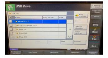
The print from USB menu is automatically populated, with support for PDF, JPEG, and TIFF formats. Users can also change settings for quantity, simplex/duplex, colour/mono, and paper size and source. Users can also navigate and print from sub-folders. However, file preview did not function.
