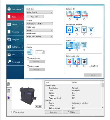
Most typical print job settings are selectable from the Basic tab, including paper type and source, duplex, EcoPrint On/ Off, quantity, and collate sets, although finishing selections such as stapling are programmable from the Finishing tab.
