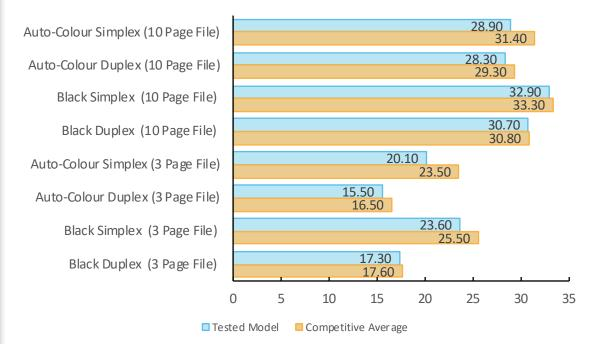
Speed is tested using Buyers Lab's proprietary 3-page and 10-page testing documents. Buyers Lab obtains the overall speed by averaging the tested speed for each run length (1, 5 and 10 sets). The unit was tested using the PCL driver.
