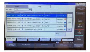
Users can view all print, scan, and copy jobs in a single list, or they can choose to view only specific types of jobs. The number of originals and numbers of sets in a job are listed, as are jobs that are complete and incomplete. The queue displays the total number of sets in a job, but not the time until job completion. Jobs can be promoted to the top or one slot at a time for maximum flexibility. However, jobs cannot be modified beyond quantity.
