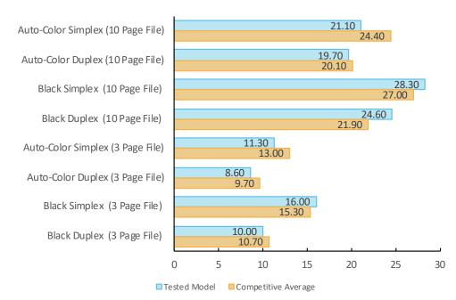
Single-set speed is tested using Buyers Lab's proprietary 3-page and 10-page testing documents. The unit was tested using the PCL driver.
