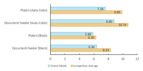
First-copy time is measured as the time it takes for a single copy to completely exit the device when a copy is made from an original placed in the document feeder and on the platen.
