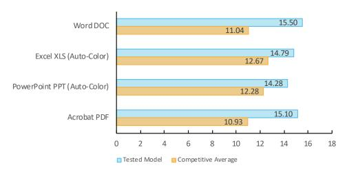
First-print time indicates the time it took to process the image and deliver a single-page test document to the output tray. The unit was tested using the PCL driver.
