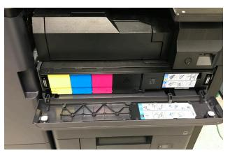
The process for replacing toner is simple and clean. Only when the container is empty will the device notify the user to open the front panel and make the replacement, helping to prevent premature replacement of toner. Guidance at the control panel is extensive and includes text, graphics, animation, and video.
