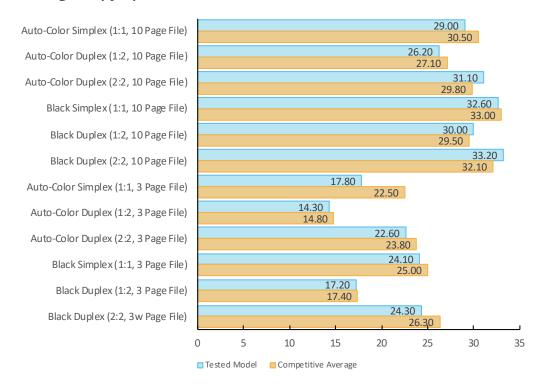
Copy speed is tested using 3-page and 10-page mixed-color and black documents. Buyers Lab obtains the overall speed by averaging the tested speed for each run length (1, 5 and 10 sets).
