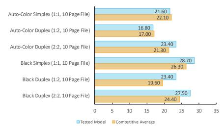
Single-set copy speed is tested using 3-page and 10-page mixed-color and black documents. Timing begins as the start button is pressed, pages are scanned through the document feeder and timing ends when the last page of a single-set of the document exits the device.
