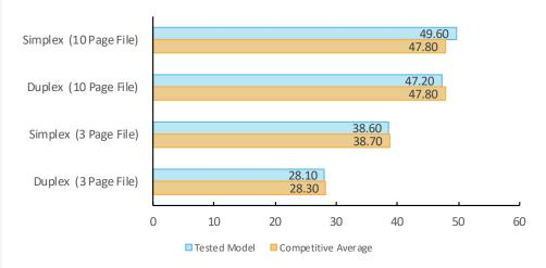
Speed is tested using Buyers Lab's proprietary 3-page and 10-page testing documents. Buyers Lab obtains the overall speed by averaging the tested speed for each run length (1, 5, 10, and 20 sets). The unit was tested using the PCL driver.
