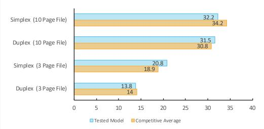
Single-set speed is tested using Buyers Lab's proprietary 3-page and 10-page testing documents. The unit was tested using the PCL driver.
