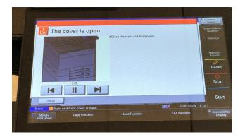
Users are also presented with an animated video to help clear misfeeds; users can let the video play or scroll through step by step using the arrows at the control panel.
