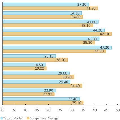
Copy speed is tested using 3-page and 10-page mixed-colour and black documents. Buyers Lab obtains the overall speed by averaging the tested speed for each run length (1, 5 and 10 sets).
