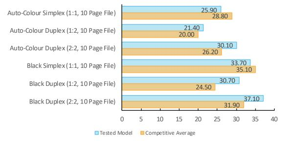
Single-set copy speed is tested using 3-page and 10-page mixed-colour and black documents. Timing begins as the start button is pressed, pages are scanned through the document feeder and timing ends when the last page of a single-set of the document exits the device.
