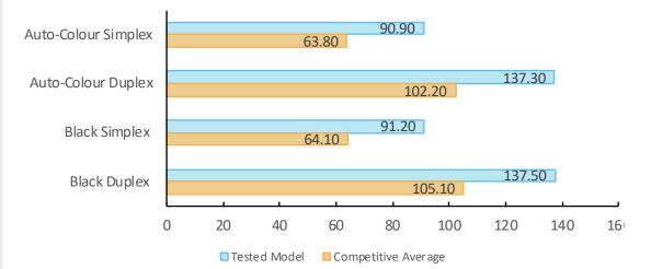
Testing is conducted with a 10-page file scanned in default mode at 300 dpi in PDF format. Tests were conducted using U.S. letter-size paper; A4 results may vary slightly.
