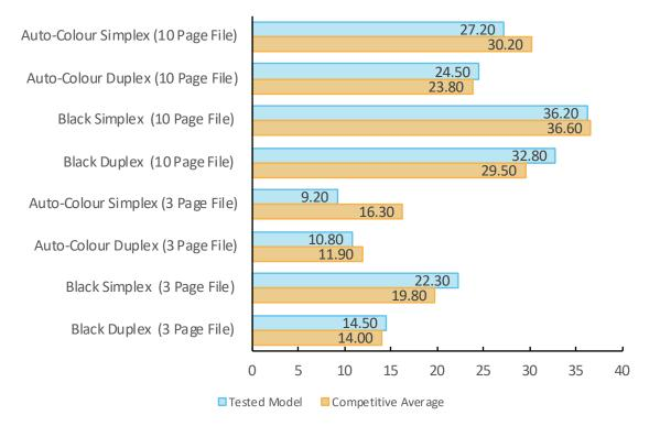
Single-set speed is tested using Buyers Lab's proprietary 3-page and 10-page testing documents. The unit was tested using the PCL driver.
