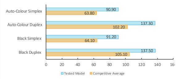
Testing is conducted with a 10-page file scanned in default mode at 300 dpi in PDF format. Tests were conducted using U.S. letter-size paper; A4 results may vary slightly.
