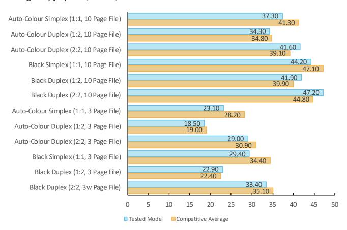
Copy speed is tested using 3-page and 10-page mixed-colour and black documents. Buyers Lab obtains the overall speed by averaging the tested speed for each run length (1, 5 and 10 sets).
