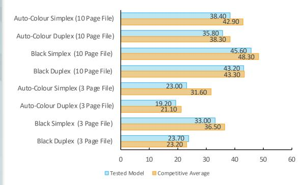
Speed is tested using Buyers Lab's proprietary 3-page and 10-page testing documents. Buyers Lab obtains the overall speed by averaging the tested speed for each run length (1, 5 and 10 sets). The unit was tested using the PCL driver.
