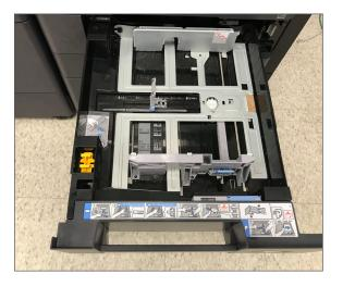
Both length and width guides slide in sync when adjusting paper size in the drawers and have blue locking tabs for easy view. The drawers also feature easy-to-see limit indicators for standard paper, envelopes, and small sizes. The soft close drawers make for no slamming of cassettes, and also pull our far enough for easy access in case of misfeed.
