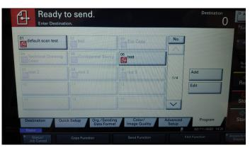
The scan and copy menus can also be customized on a user by user basis by adding up to six shortcuts for functions that can be found under the System Menu button on the Home screen taskbar. In addition, up to 50 job programs can be saved within the scan or copy menus, or even on the Home screen, to streamline workflow of commonly run jobs. The order of features on the home page and the Quick Setup tab can be prioritized as well.
