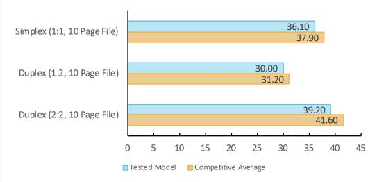
Single-set copy speed is tested using 3-page and 10-page mixed-colour and black documents. Timing begins as the start button is pressed, pages are scanned through the document feeder and timing ends when the last page of a single-set of the document exits the device.
