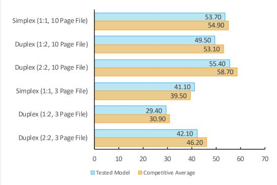
Copy speed is tested using 3-page and 10-page mixed-colour and black documents. Buyers Lab obtains the overall speed by averaging the tested speed for each run length (1, 5, 10, and 20 sets).
