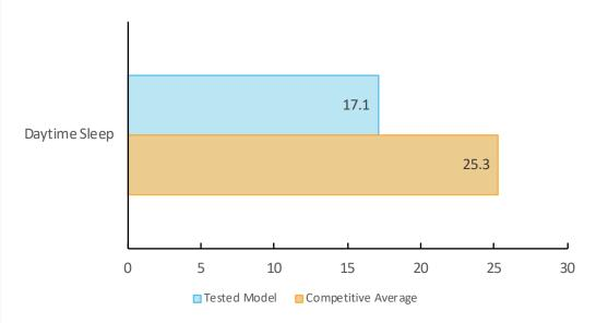
Recovery time in seconds indicates the time it took to warm up, process the image and deliver a single-page test document to the output tgrey. The unit was tested with the PCL driver.
