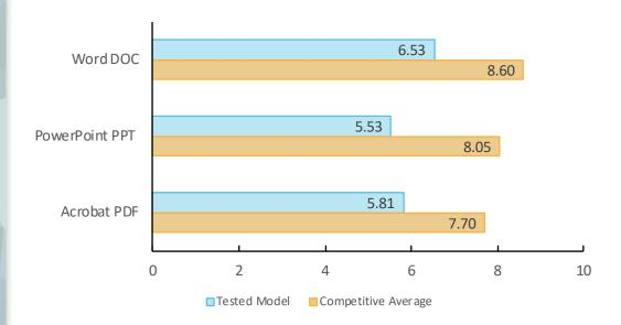
First-print time indicates the time it took to process the image and deliver a single-page test document to the output tgrey. The unit was tested using the PCL driver.
