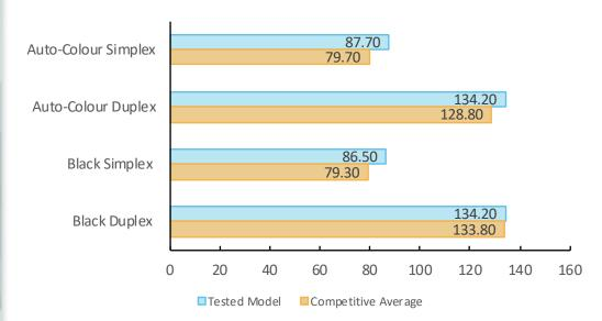
Testing is conducted with a 10-page file scanned in default mode at 300 dpi in PDF format.
