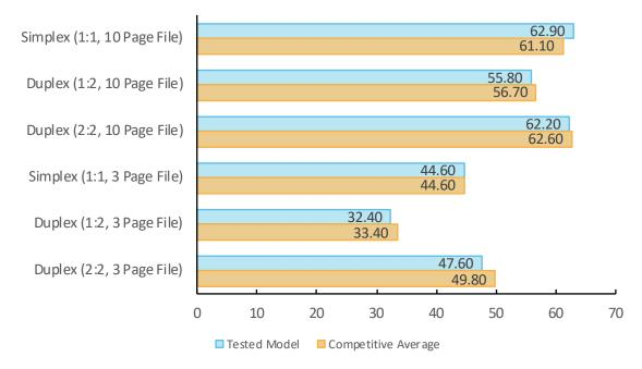
Copy speed is tested using 3-page and 10-page mixed-colour and black documents. Buyers Lab obtains the overall speed by averaging the tested speed for each run length (1, 5, 10, and 20 sets).
