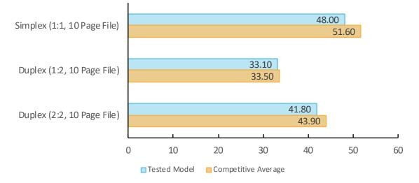
Single-set copy speed is tested using 3-page and 10-page mixed-color and black documents. Timing begins as the start button is pressed, pages are scanned through the document feeder and timing ends when the last page of a single-set of the document exits the device.
