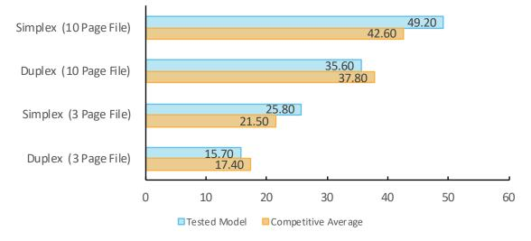
First-print time indicates the time it took to process the image and deliver a single-page test document to the output tray. The unit was tested using the PCL driver.
