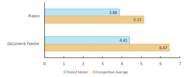
First-copy time is measured as the time it takes for a single copy to completely exit the device when a copy is made from an original placed in the document feeder and on the platen.
