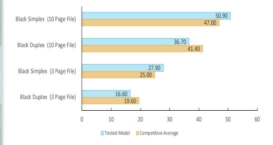
Single-set speed is tested using a Buyers Lab's proprietary 3-page and a 10-page testing document. The unit was tested using the PCL driver.
