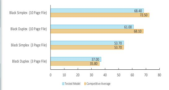
Speed is tested using Buyers Lab's proprietary 3-page and 10-page testing document. Buyers Lab obtains the overall speed by averaging the tested speed for each run length (1, 5, 10, and 20 sets). The unit was tested using the PCL driver.
