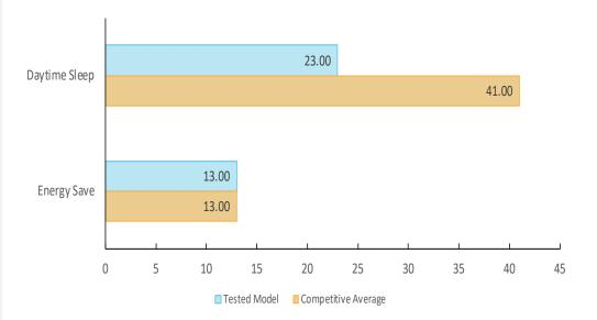
Recovery time in seconds indicates the time it took to warm up, process the image, and deliver a single-page test document to the output tray. The unit was tested with the PCL driver.
