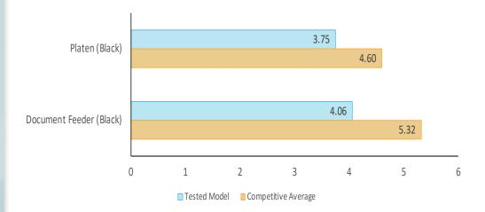
First-copy time is measured as the time it takes for a single copy to completely exit the device when a copy is made from an original placed in the document feeder and on the platen.
