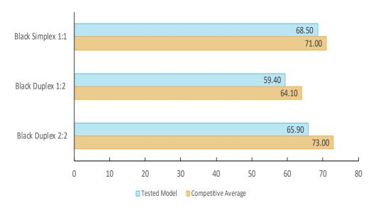
Copy speed is tested using Buyers Lab's proprietary 10-page testing document. Buyers Lab obtains the overall speed by averaging the tested speed for each run length (1, 5, 10, and 20 sets).
