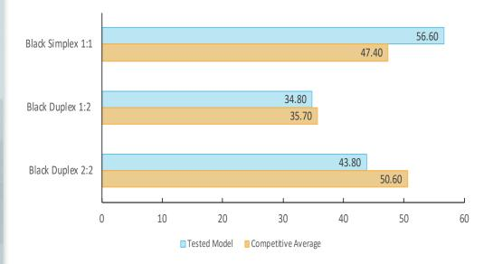
Single-set copy speed is tested using Buyers Lab's proprietary 10-page testing document. Timing begins as the start button is pressed, pages are scanned through the document feeder and timing ends when the last page of a single-set of the document exits the device.
