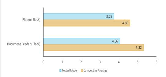
First-copy time is measured as the time it takes for a single copy to completely exit the device when a copy is made from an original placed in the document feeder and on the platen.
