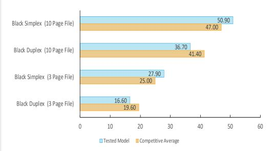
Single-set speed is tested using a Buyers Lab's proprietary 3-page and a 10-page testing document. The unit was tested using the PCL driver.
