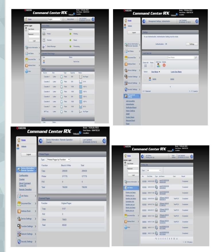
The web user interface is easy to navigate, with functions clearly labelled and selectable. Job history can be exported from the web user interface. Access codes can be assigned so that print, scan, and copy usage can be restricted and tracked by user and group. Detailed counters and printing and sending logs are also provided. However, administrators cannot remotely add or edit destinations from the LDAP servers. (US model pictured)
