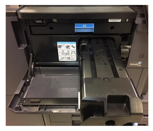
The process for replacing toner is simple and clean. Only when the container is empty will the device notify the user to open the front panel and make the replacement, helping to prevent premature replacement of toner.
