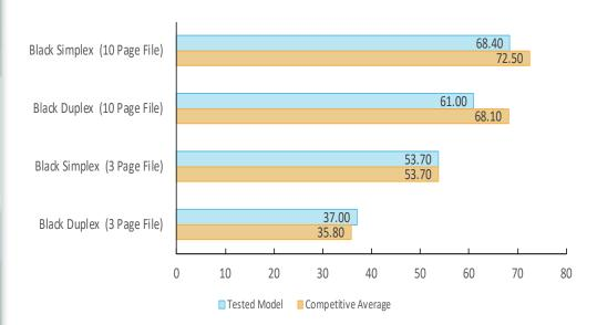
Speed is tested using Buyers Lab's proprietary 3-page and 10-page testing document. Buyers Lab obtains the overall speed by averaging the tested speed for each run length (1, 5, 10, and 20 sets). The unit was tested using the PCL driver.
