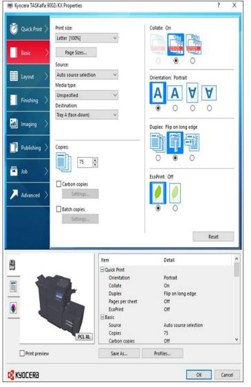
Most typical print job settings are selectable from the Basic tab, including paper type and source, duplex, EcoPrint On/Off, quantity, and collate sets, although finishing selections such as stapling are programmable from the Finishing tab.
