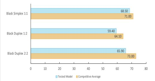
Copy speed is tested using Buyers Lab's proprietary 10-page testing document. Buyers Lab obtains the overall speed by averaging the tested speed for each run length (1, 5, 10, and 20 sets).
