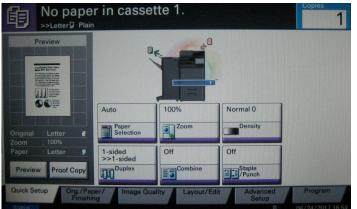
Most of the selections for a typical copy job can be accessed from the Quick Setup tab, including duplex, paper source, colour mode, reduction/enlargement, and finishing. The control panel can also be angled in multiple positions. Each user can also customize the location of each key on the main page, add settings to the main screen, and select their default home screen and language.
