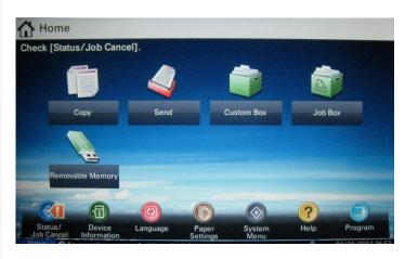
Up to 50 scan jobs can be saved as job programs within the scan menu or even on the Home screen to streamline workflow of commonly run jobs.
