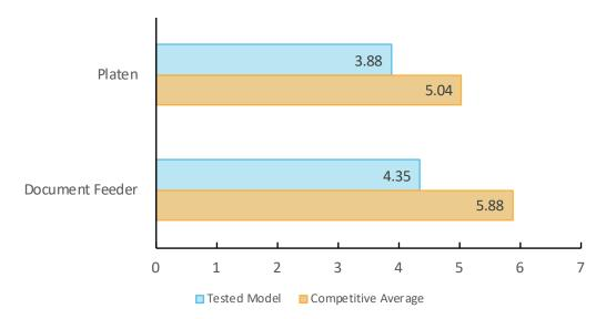
First-copy time is measured as the time it takes for a single copy to completely exit the device when a copy is made from an original placed in the document feeder and on the platen.
