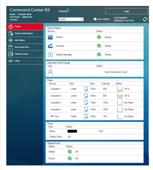
The main screen of the web user interface, Command Center RX, includes notifications and gauges on the status of the device including device state, and paper drawers and consumables in percent increments. Print, scan, and copy usage can be restricted and tracked by user and group. Up to three event reports can be set up and schedulled for when to add paper, add toner, cover open, paper jam, low toner, waste toner replacement, and other errors.
