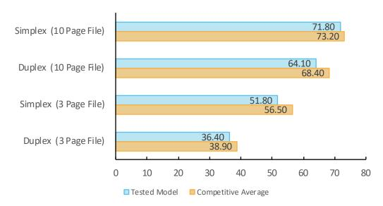
Speed is tested using Buyers Lab's proprietary 3-page and 10-page testing documents. Buyers Lab obtains the overall speed by averaging the tested speed for each run length (1, 5, 10, and 20 sets). The unit was tested using the PCL driver.
